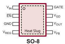
Backside on the SO-8 package is at ground potential and may be connected to ground or left unconnected.
